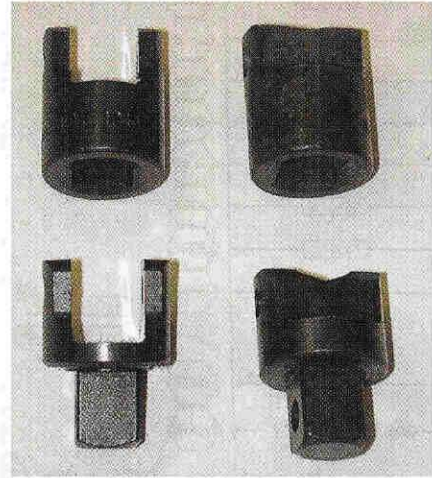
The U-joints Abrasive-Form tested were made of 4140 steel.
